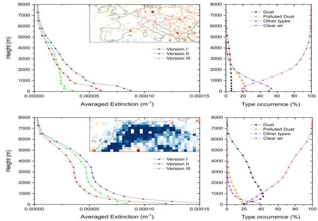
The dust product of BEYOND is provided with a vertical resolution of 60m. The LIVAS BEYOND products are currently used as the Reference Atmospheric Model (RAM) by ESA for simulation tests in hardware and software level of future lidar missions like ADM-Aeolus and EarthCARE Earth Explorers.
