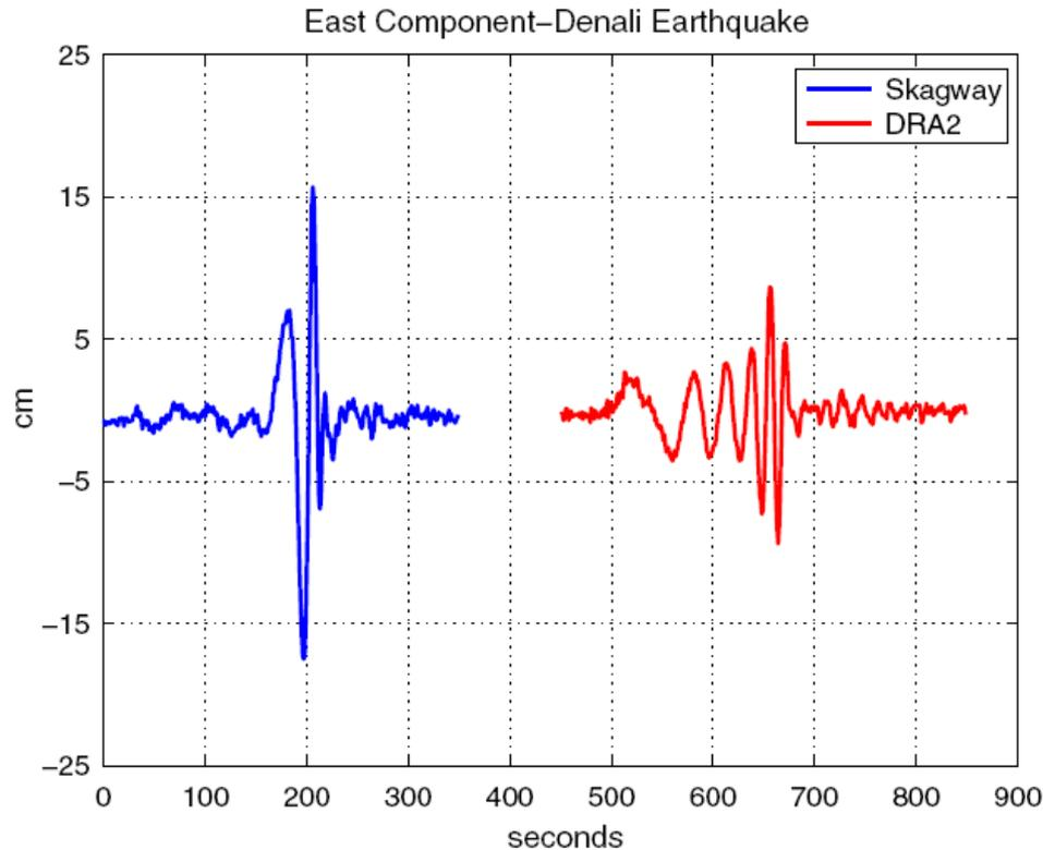
**Fig. 2** East component GPS displacement records for a Skagway site and DRA2. These GPS receivers were located over 700 and 2,200 km, respectively, from the Denali epicenter. The difference in arrival times for the seismic displacements reflects the additional time it took the surface waves to travel the 1,500 km between Skagway and DRA2
