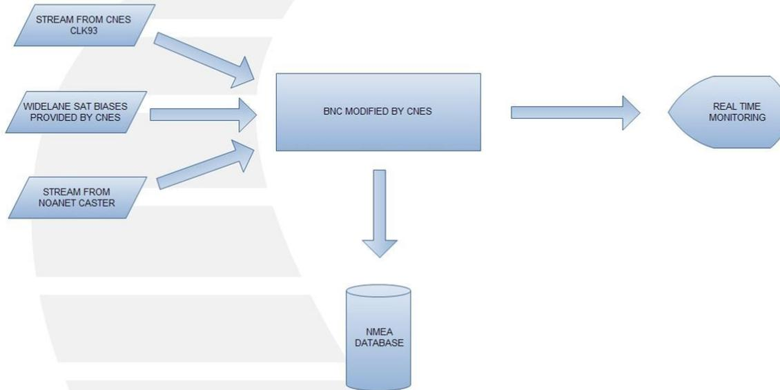
The PPP (Precise Point Positioning) processing technique is used to detect offsets in XYZ positions of GNSS stations in the Ionian Sea and Santorini Island, where tsunami hazard is high. PPP works on a single station, double-frequency, basis, continuously using the real-time RTCM v3.0 stream. PPP is a method to determine the exact coordinates of a single point using code or phase measurements with precise clocks and orbits.
