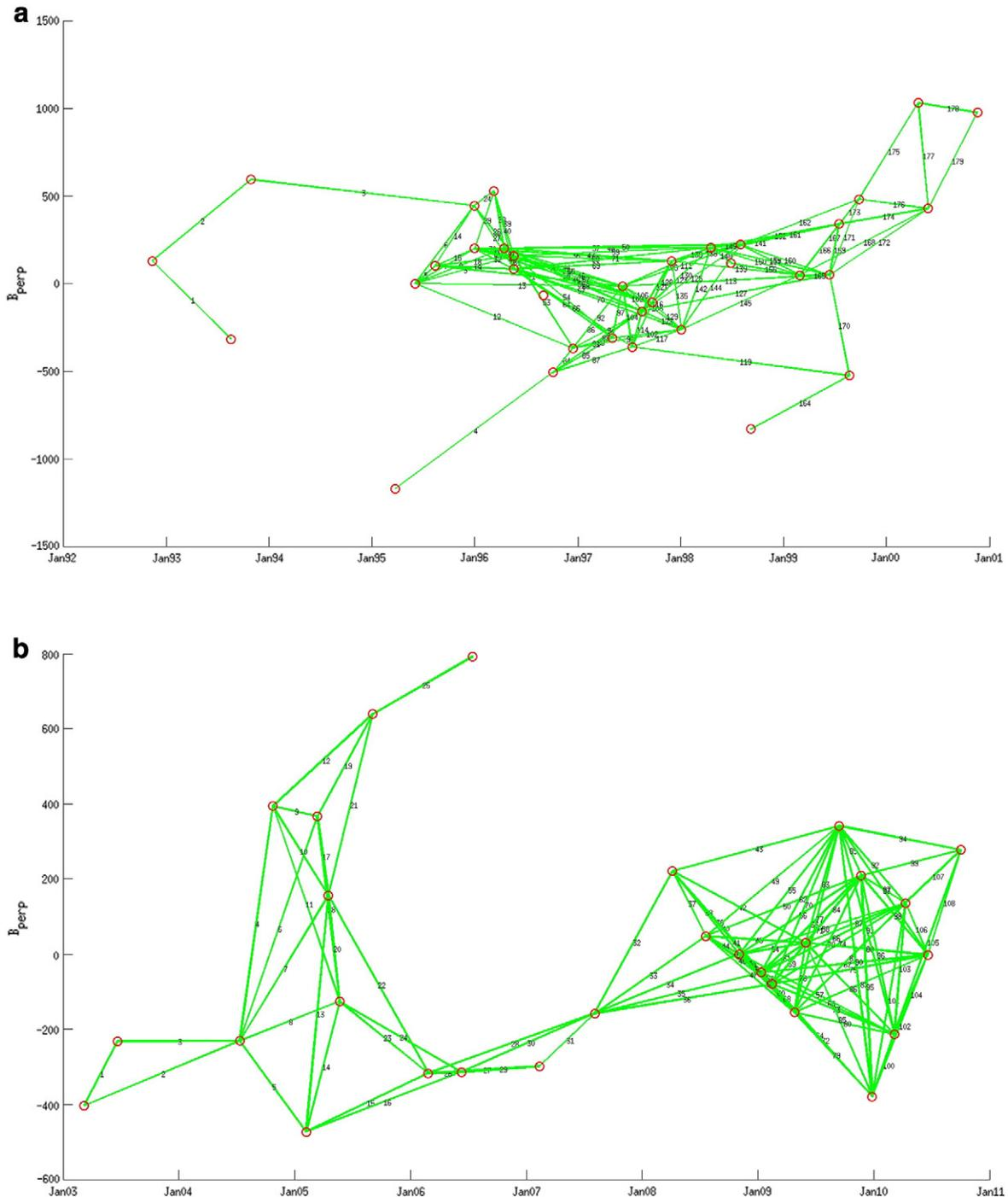
Fig. 7. a Connection graph showing the Differential Interferograms created for the SBAS technique for the ERS dataset b Connection graph showing the SLC network created for the SBAS technique for the ENVISAT dataset.
