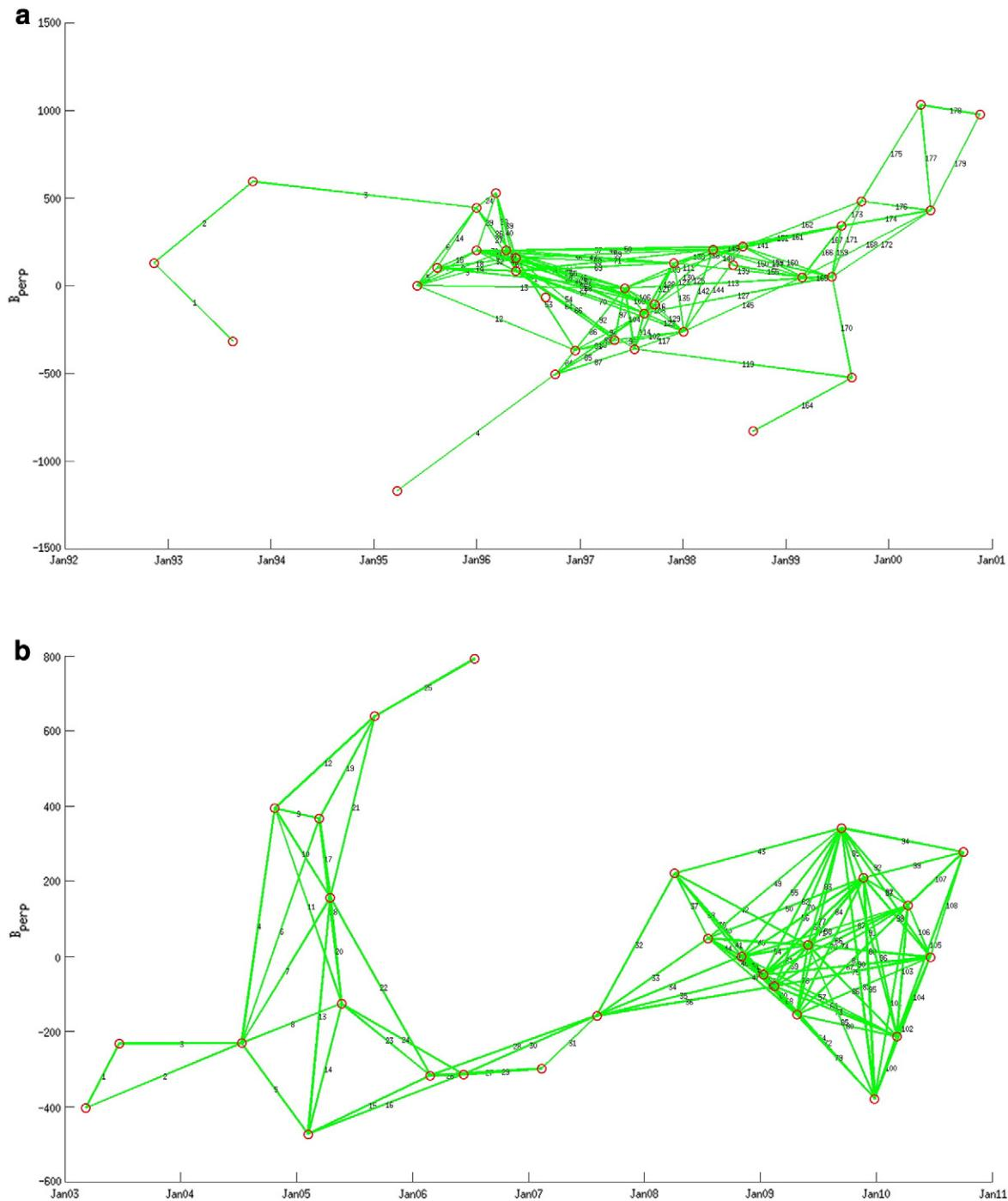
**Fig. 7.** a Connection graph showing the Differential Interferograms created for the SBAS technique for the ERS dataset b Connection graph showing the SLC network created for the SBAS technique for the ENVISAT dataset.
