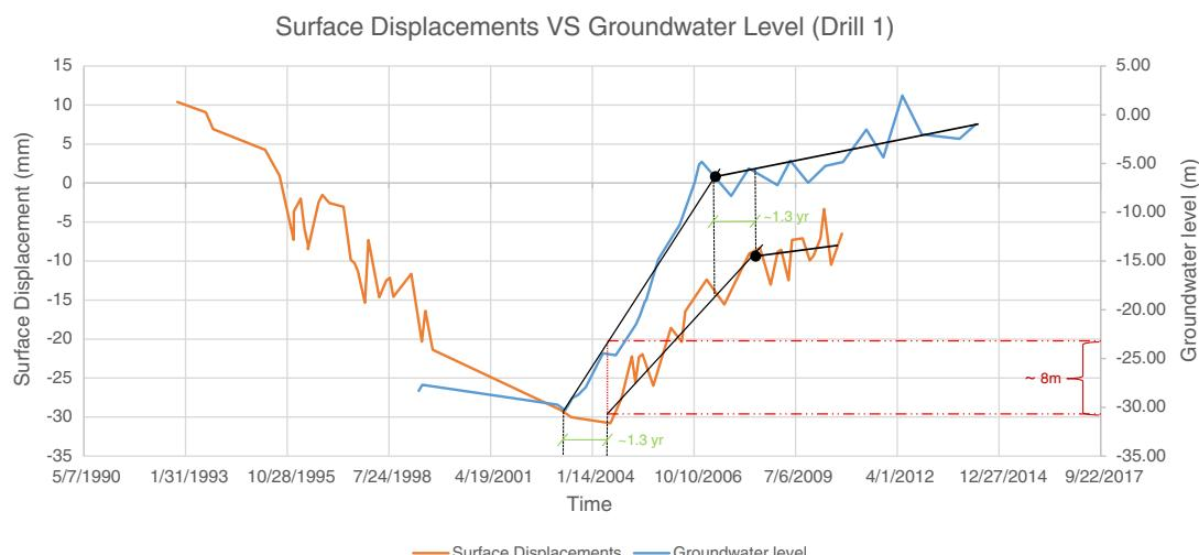
**Fig. 10.** Graph comparing the ground water level variations at Drill 1 with the surface deformation time series at a nearby data point produced by the SAR analysis.
