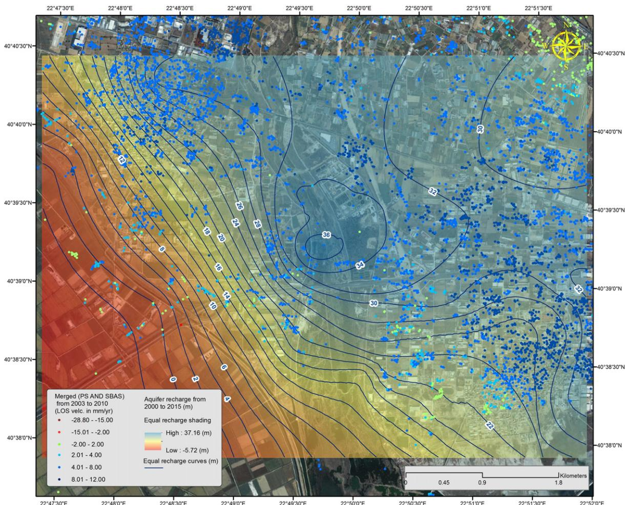
**Fig. 5.** Image presenting the groundwater recharge (in m) between June 2000 and June 2015. The dots are SAR data indicating displacements along LOS in mm/year (2003–2010). Positive values of the aquifers recharge contour indicate uplifting of the ground water level.
