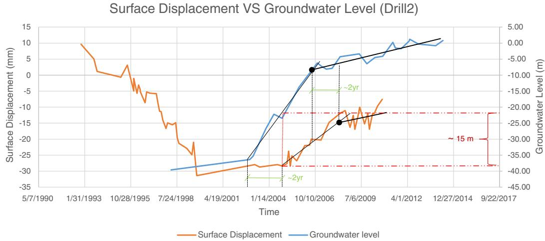
**Fig. 11.** Graph comparing the ground water level variations at Drill 2 with the surface deformation time series at a nearby data point produced by the SAR analysis.
