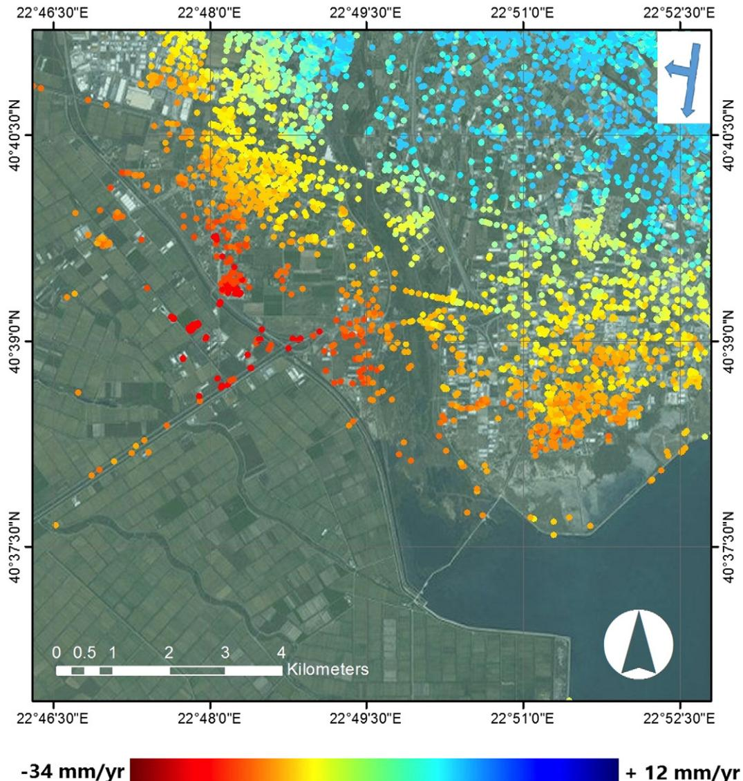
**Fig. 8.** Velocities from 1993 to 2000 as derived by the analysis of ERS 1 & 2 data. During this time period the study area was subsiding with a rate of 20 mm/year. The large arrow depicted in the inset in the upper right, shows the direction of the descending path and vertical smaller arrow shows the line of sight direction of the satellite.
