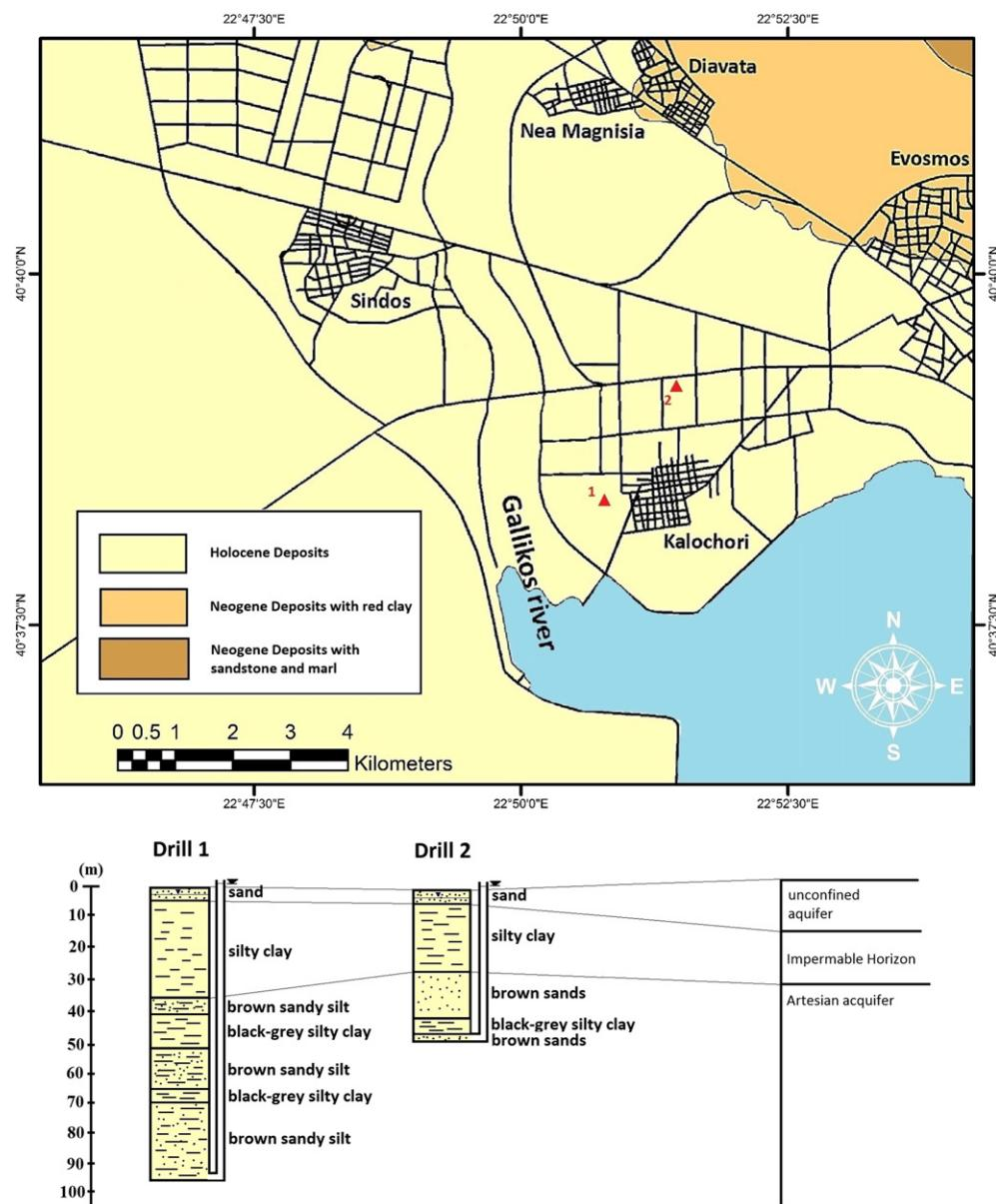
**Fig. 4.** Geological map of the area (modified after IGME, 1978 and Raspini et al., 2014). With red triangles two drills are denoted. Below the map the Drills' logs and the aquifers succession are presented. Drill loggings are from Andronopoulos et al. (1990). (For interpretation of the references to colour in this figure legend, the reader is referred to the web version of this article.)
