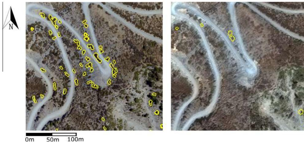
**Fig. 13.** The effectiveness of the evaluation criteria in rejecting false changes which arise due to the difference in image sharpness between  $Im^{UAV}$  (left) and  $Im^{sat}$  (right). The  $PCC$ 's (marked on the left image) were refined via the SRG algorithm into  $Reg^{UAV}$ 's. The evaluation criteria help in rejecting many homogeneous regions as no change; finally, the rest of them are confirmed as changes (marked on the right image).
