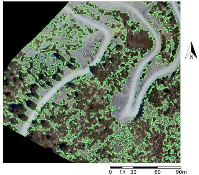
Fig. 4. The image segmentation result. The contour encircles the “high saturation” class while the rest belongs to “bare ground” class.
