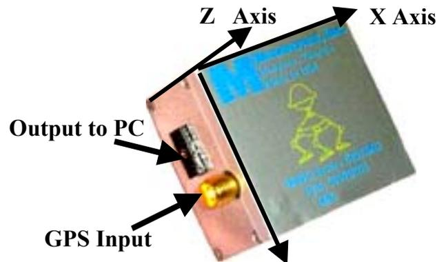
**Table 3.** MIDG II Inertial Navigation Device characteristics
