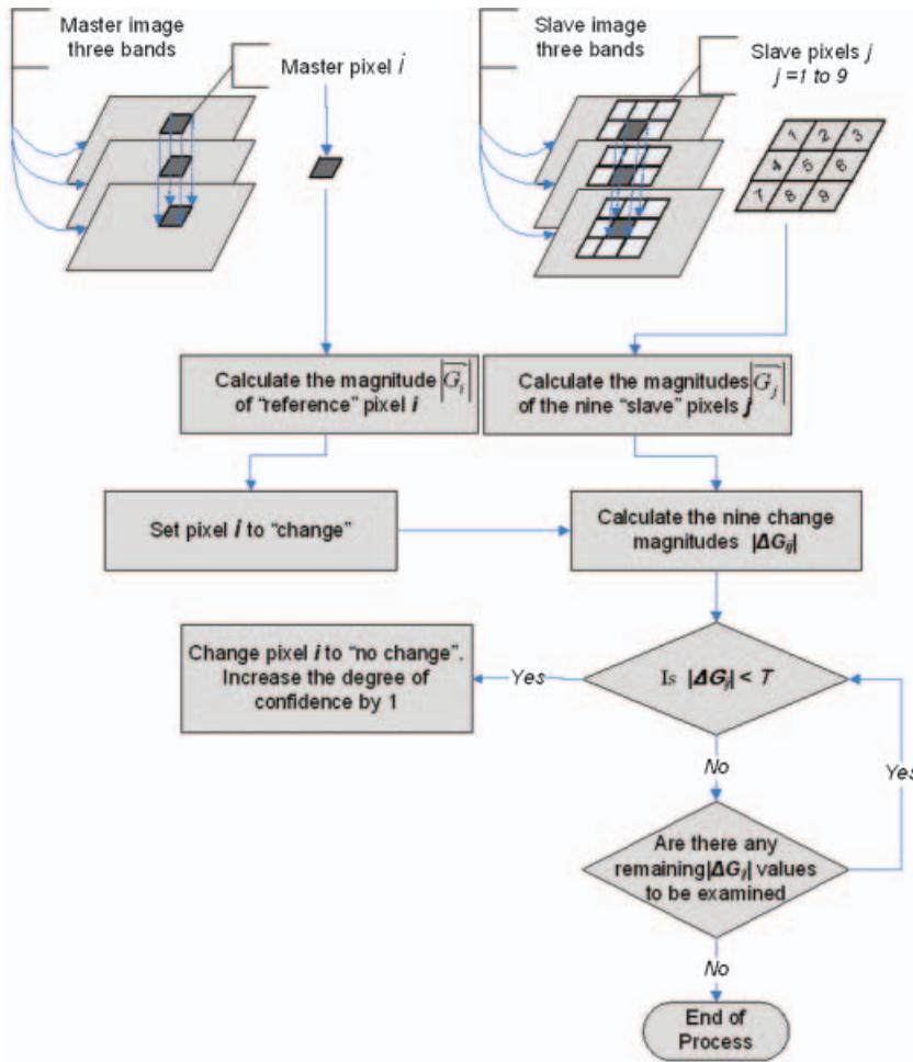
Figure 2. Flowchart of the kernel-based thresholding method to map change/no-change pixels.
