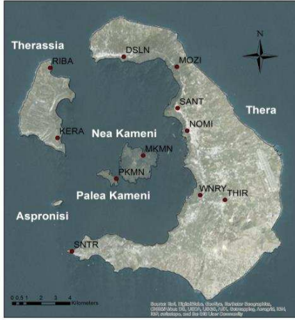
Figure 8. Santorini volcanic complex map. Red dots shows the GPS network of permanent stations
