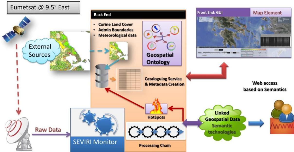
Figure 1. Fire monitoring service architecture.
