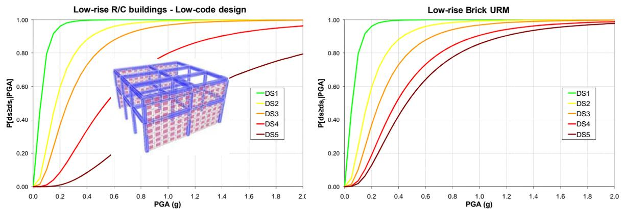
**Figure 3.1.** Fragility curves in terms of PGA for low code, low rise with frame system (left) and low rise, brick URM buildings (right)
