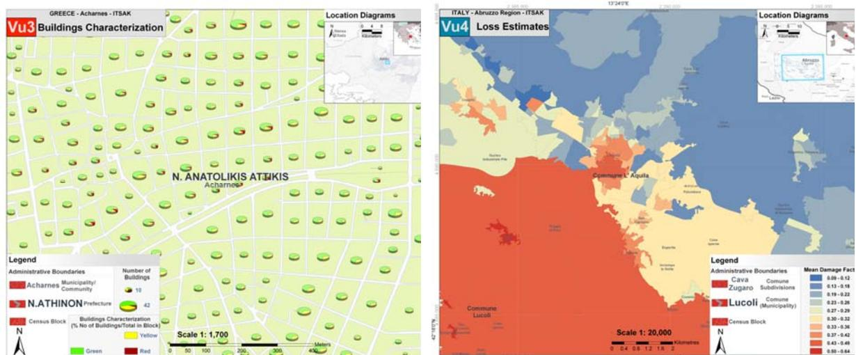
**Figure 4.2.** Predicted distribution of post-earthquake damage distribution in terms of green-yellow-red tagging for Athens (left) and Mean Damage Factor for L’Aquila (right)
