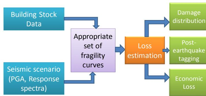
**Figure 5.1.** The AUTH/ EPPO-ITSAK loss estimation procedure scheme
