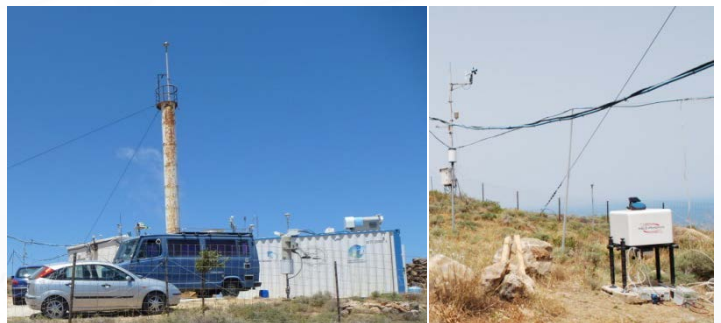
The 3 lidars (mobile EMORAL (blue van) POLLY-XT (container) and HALO wind lidar (right))
