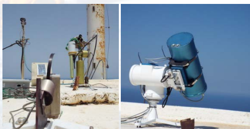
CIMEL and UV-MFR sun-photometers (left) and PSR radiometer (right)
